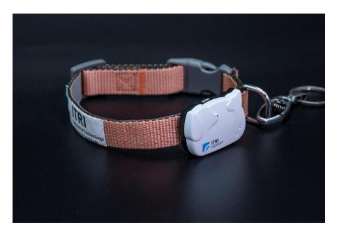
Introduced at CES 2022, ITRI is presenting **iPetWeaR**, the world's first smart wearable device using contactless micro-physiological radar sensing technology for pet health monitoring. This sensor package continuously monitors the health parameters of pets including heart rate, respiration, and activity to identify their health status via user-friendly operation.
